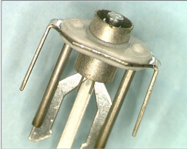
Philips 0,65 Watt I cathode unit, used as base for LAD top-layer Scandate cathode
