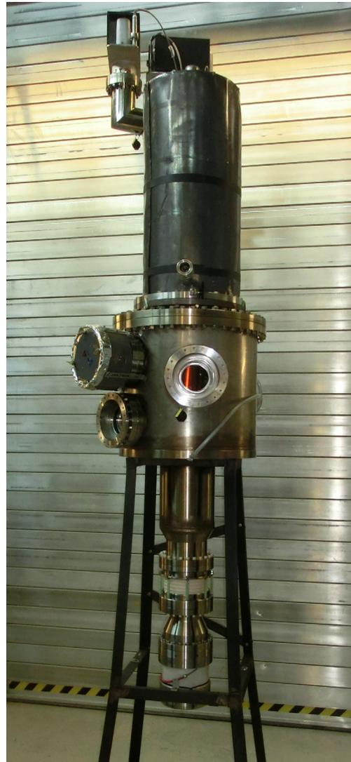
Fig. 1.1.1: EU 1 MW short-pulse gyrotron prototype for ITER.
