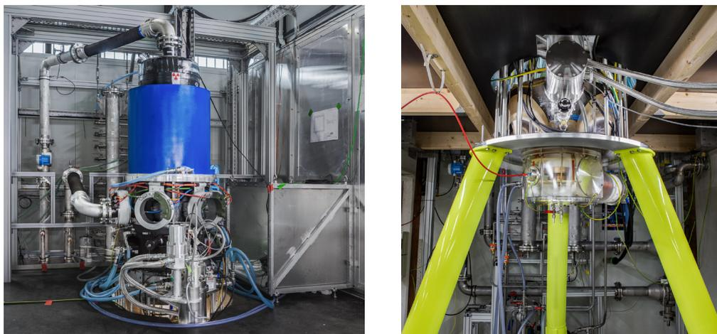
Fig. 1.7.1: TH1511 installed in the super conducting magnet (left), bottom part of the gyrotron with support structure, HV isolation oil tank and magnet (right).
