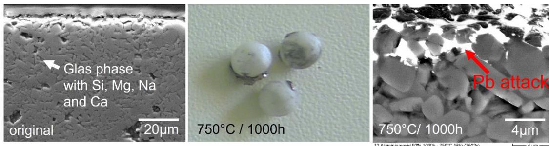
Fig. 2.3.3 : Alumina 92%: cross section of the original material (left), samples after 1000h at 750°C in Pb (middle) and
