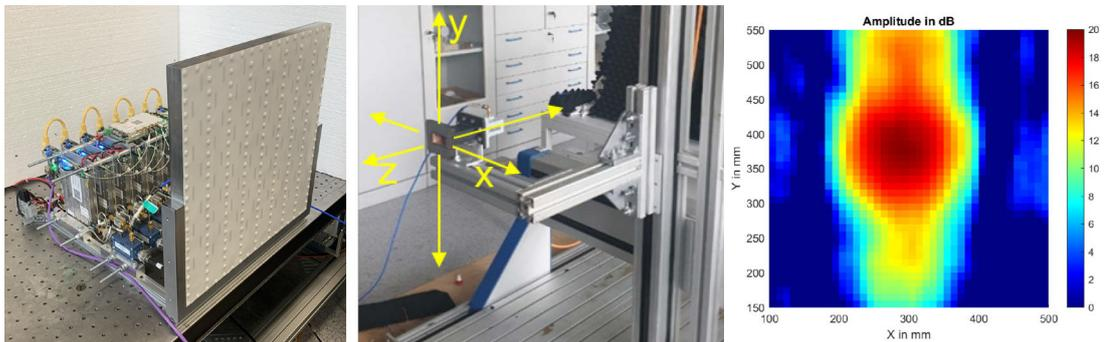
Fig. 4.5.1: Test stand for measuring antenna characteristics using digital signal generators with phase shifting and the slotted waveguide array antenna (left) and a WR159 receiving antenna probe fixed to a xyz positioning stage (middle). Measured zero phase-shift x-y plane field profile at a distance of 50 cm to the antenna. Most of the energy is nicely focused in the center (right).
