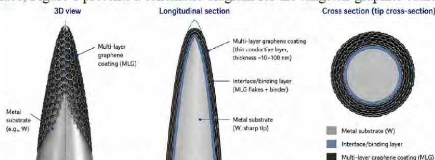
Figure 1: Schematic diagram for a tungsten-graphite electrode apex.
