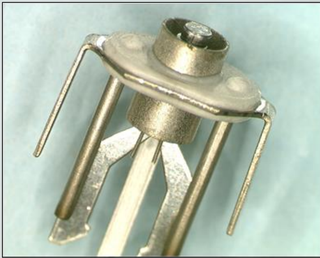
Philips 0,65 Watt I cathode unit, used as base for LAD top-layer Scandate cathode
