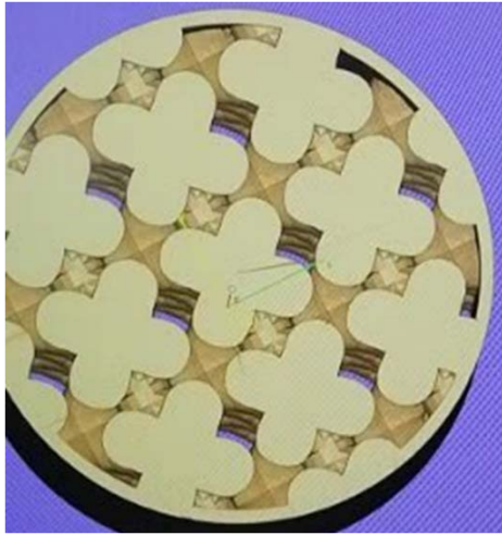
3D printing grid structure model with the porosity of 25% in the tungsten matrix
