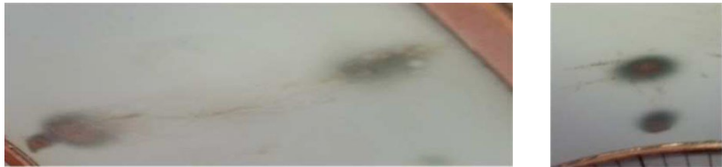
Surface discharge traces on alumina ceramics
