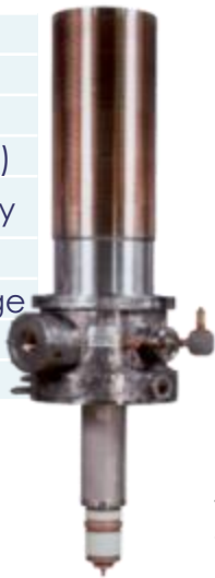
The 140 GHz gyrotron for the stellarator W7-X
