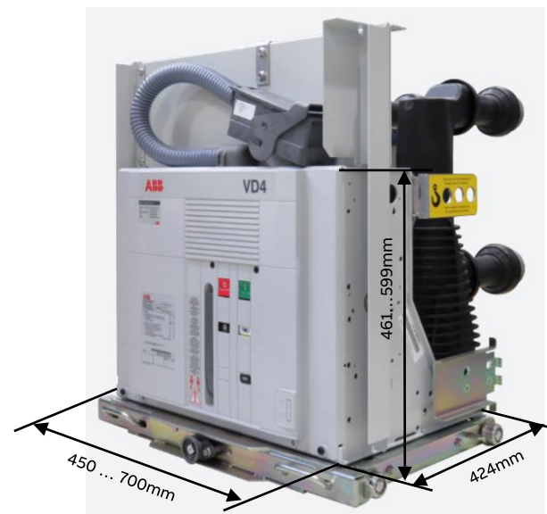
Vacuum Circuit breaker type VD4: 12kV, 2000A, 40kA
