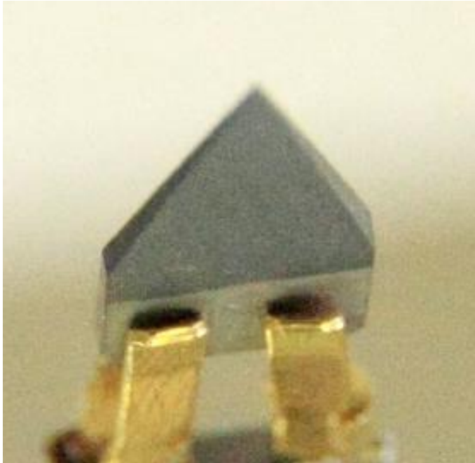
Specimen base in cross section — 0.1 by 0.6 cm.
