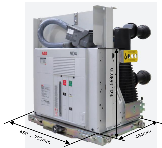
Vacuum Circuit breaker type VD4: 12kV, 2000A, 40kA
