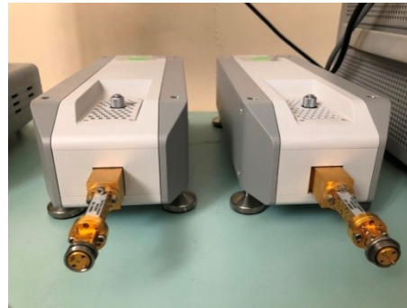
Rx/Tx frequency converters ZVA-Z260 (170-260 GHz), R&S, Germany
