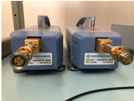
Rx/Tx frequency converters ZVA-Z170 (110-170 GHz), R&S, Germany
