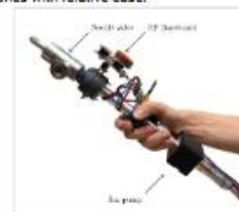
Miniature quadrupole mass spectrometer fully controlled by presented system
