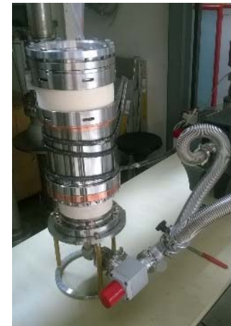
MIG with anti-emissive coated emitter edge rims
